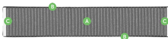
Photomicrograph cross-section of an Enovix 3D cell shows laser-patterned electrodes and separators vertically stacked within a stainless-steel constraint (source: Enovix Corporation)
