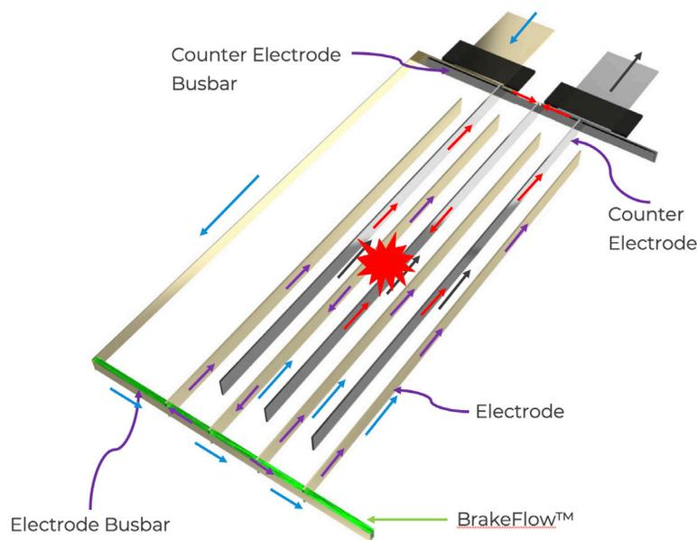
*BrakeFlow—a system that includes a resistor engineered with a set value—at the electrode-busbar junction (green). In the event of an internal short circuit (red), BrakeFlow regulates current flux from other areas of the battery to the short. This limits the flow of current and reduces the rate of heating.*
