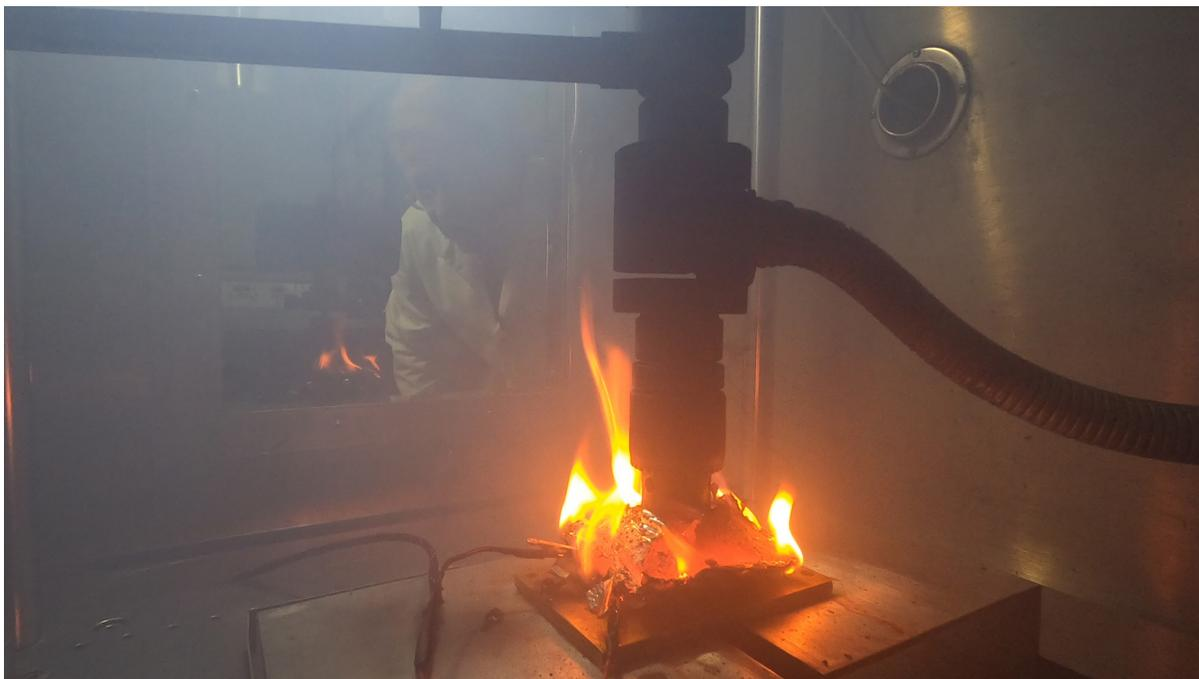
*Commercial cell phone battery succumbs to thermal runaway in a nail penetration testing machine.*
